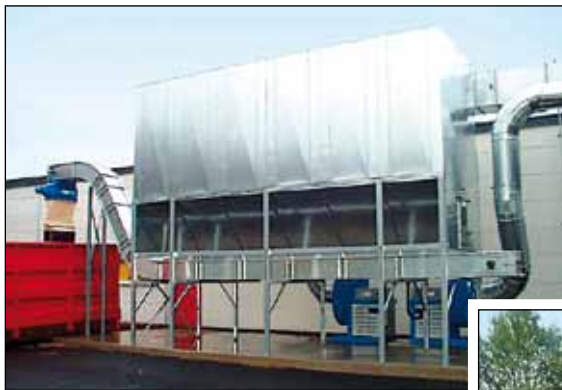
Aagaard chip conveyor filter.
